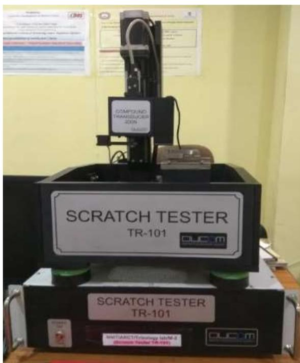
Fig.9: Test setup of Scratch Tester
