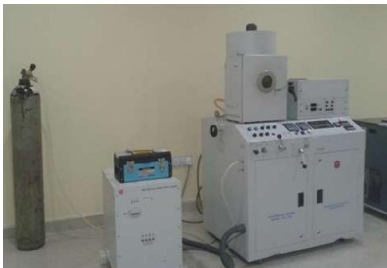
Fig.7: Thermal/E-beam PVD Coating Unit
